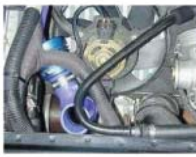
Fit hose "T" piece and valve
